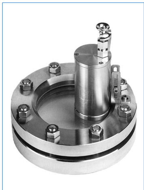
Sightglass light fitting type EdelEx 20 dH Sch K1, 20 W, 24 V, Ex d IIC T4, Ex tD A21 IP65 T130°C, Ex II 2 G + D, mounted onto circular sightglass to DIN 28120, PN 10, DN 125.
